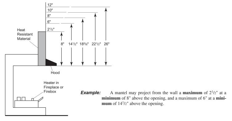
Figure 8 - Minimum Mantel Clearance with Hood - All Models
